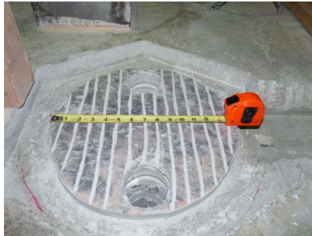
Figure 4.27: Epoxy Pad Modification for HCHP-UHPC Specimen
