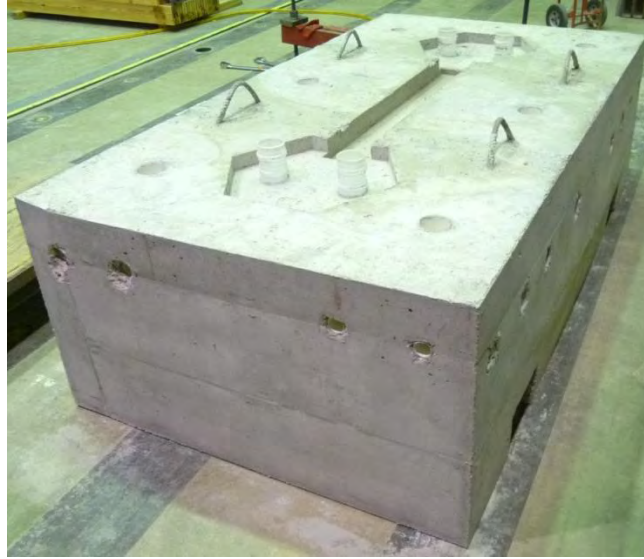
Figure 4.22: In-Plane Test Foundation Block
