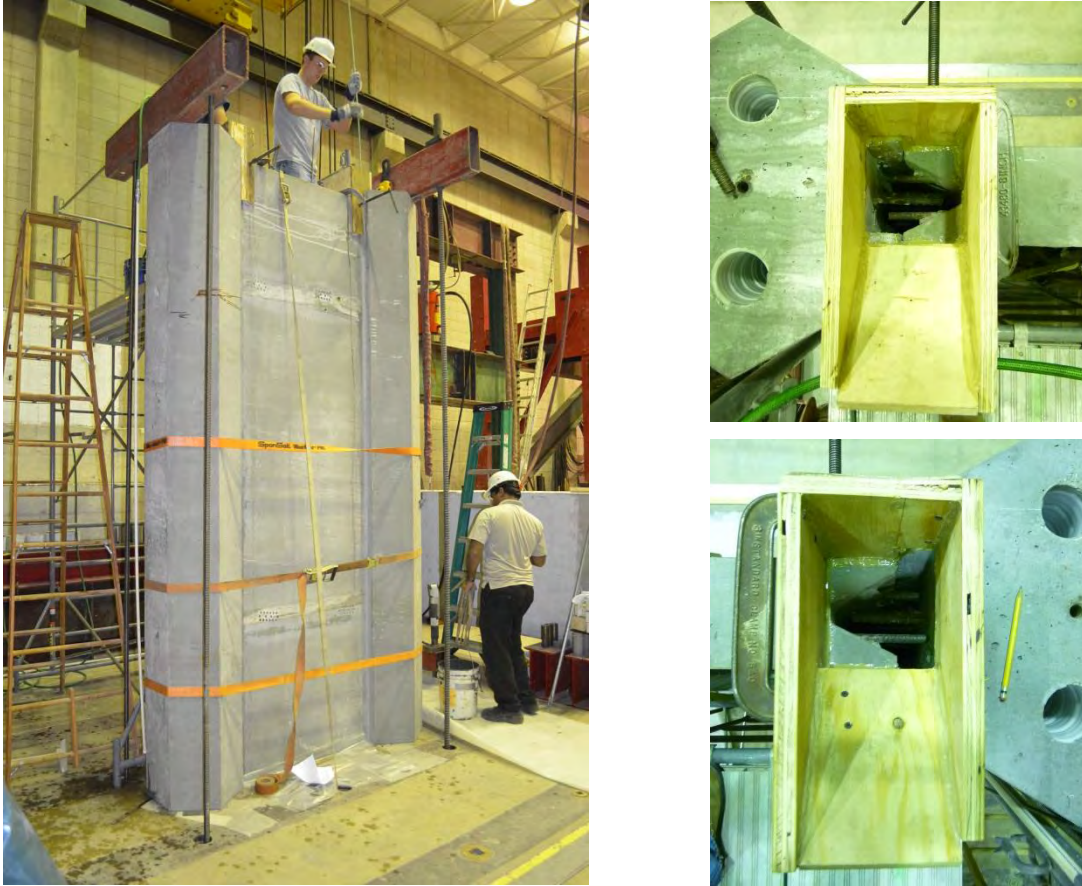
Figure 4.26: UHPC Wet Joint Specimen Assembly
