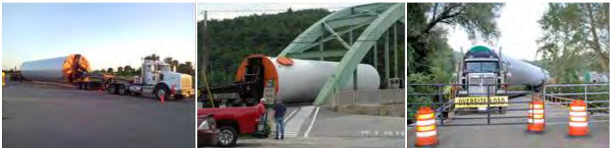
Figure 1.4: Transportation of steel tower segments and associated challenges (Karkos, 2010)
