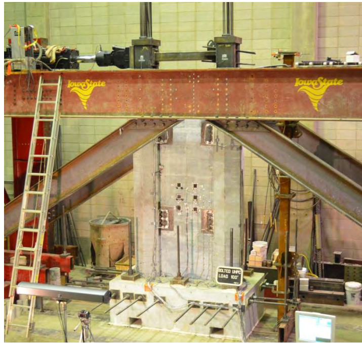
Figure 4.29: HCUP-BC Test Configuration
